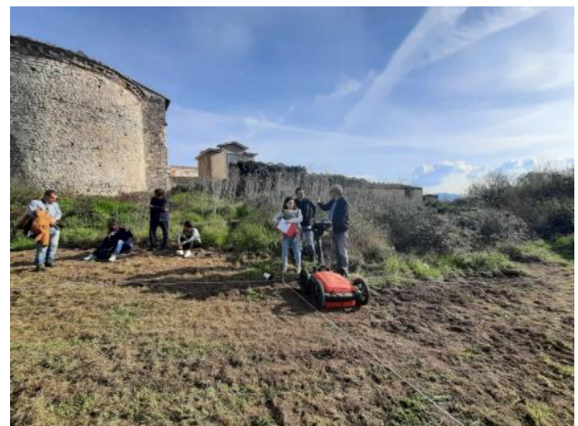
Fig. 3. GPR data acquisition in Montebuono (Area B).
